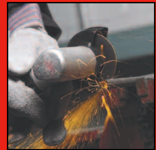
Cutting a piece of steel tubing to length.
